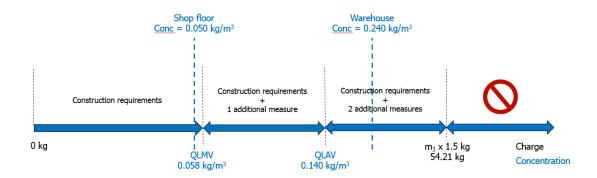
As shown in the diagram above Conc is above QLAV (quantity limit with additional ventialtion) so two additional measures are required in the warehouse. The simplest measures would be a detector and alarm plus mechanical ventilation. The alarm must provide a warning (audible and visible) at least inside the warehouse.
