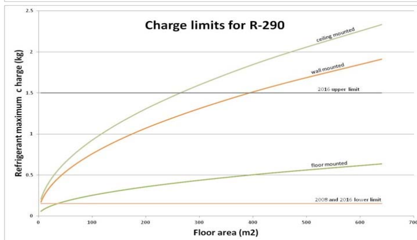
Figures 1a and 1b Charge limits for human comfort according to EN 378 Part 1 Annex C.2
